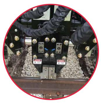
Anchors are spread to a pre-determined width and do not have to be removed then reapplied saving time and anchor replacement costs.
