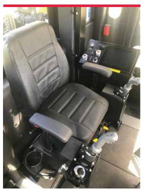
Comfortable climate controlled cab design features electronic console with joystick workhead controls.
